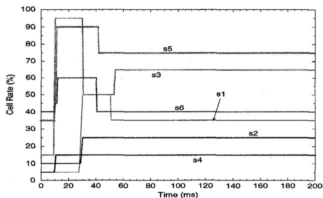
Figure 5: The cell rates of all connections for the generic fairness network configuration.
