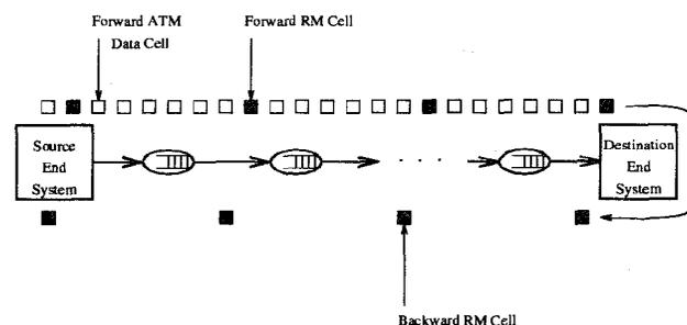
Figure 3: ABR flow control mechanism for a connection.
